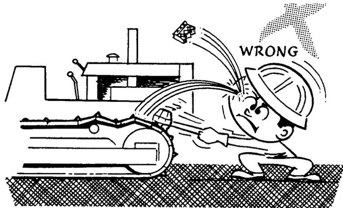
Eye injuries are one of the most common types of injuries caused by improper use of hammers. And anybody who has clobbered his thumb with a hammer on a cold day can verify the pain that this simple tool can cause!
