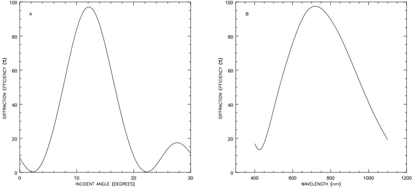
**Figure 2.** The angular and wavelength bandwidth Bragg envelopes for a theoretical 600 l/mm grating designed for 1<sup>st</sup> order operation at 700 nm. **A.** Angular bandwidth Bragg envelope. **B.** Wavelength bandwidth Bragg envelope.
