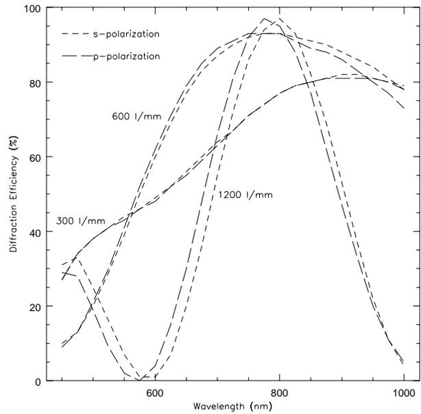
**Figure 4.** Rigorous coupled-wave prediction for the diffraction efficiency of three different gratings designed for first order operation at 790 nm. Both s and p polarization states are shown. Material and reflection losses are not included.
