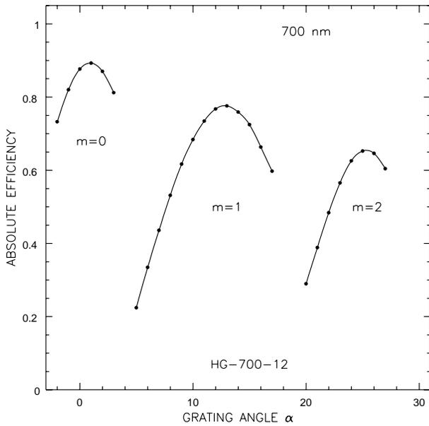
**Figure 5.** Absolute efficiency of the 600 l/mm VP grating for unpolarized light as a function of incident angle and diffracted order ( $m=0,1,2$ ) for 700 nm. Material and reflective losses are included.
