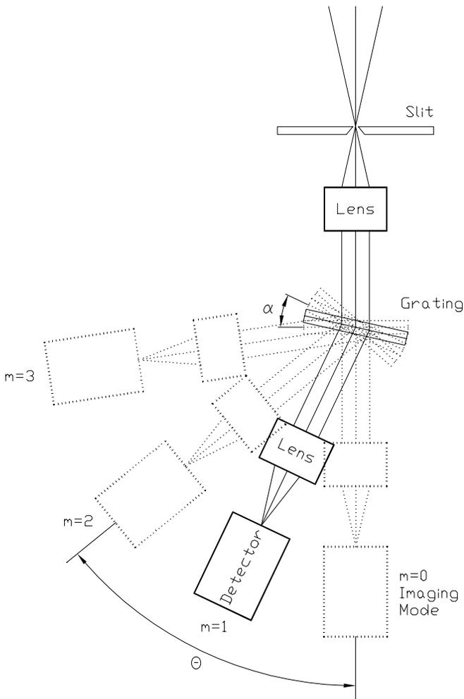
**Figure 10.** Schematic of a tunable spectrograph concept in which the camera axis angle ( $\theta$ ) and grating angle ( $\alpha$ ) are allowed to tilt in order to change the order of diffraction or to peak up the efficiency of the desired wavelength.
