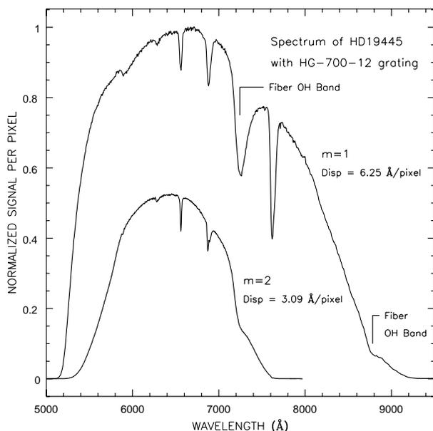
**Figure 9.** Stellar spectra obtained in first and second orders of diffraction.. The units of the ordinate axis were selected to remove confusion of the two curves but give the false impression that the 2<sup>nd</sup> order spectrum has a factor of two lower signal.
