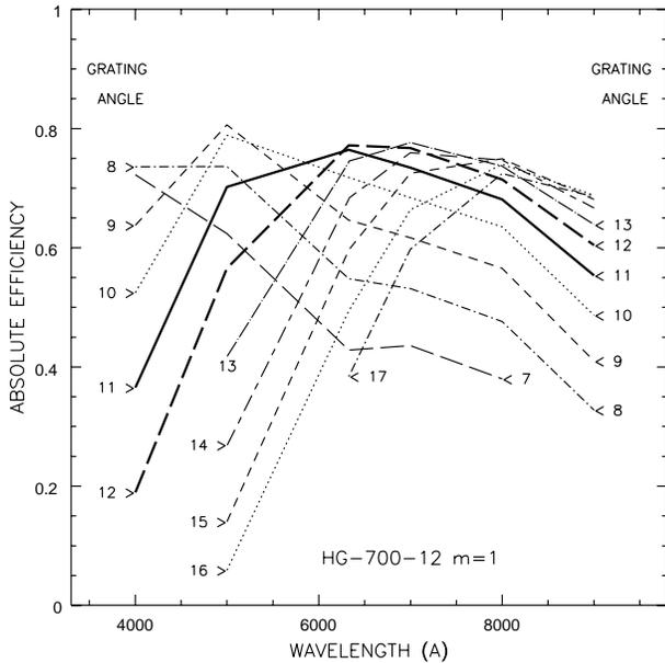
**Figure 7.** Efficiency envelope of the 600 l/mm VP grating as a function of incident angle for first order diffraction. Grating tilts of 11 and 12 degrees give the best overall efficiency in the design bandwidth from 500 to 900 nm.
