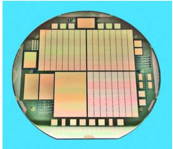
*This mechanical silicon wafer incorporates three OTAs (the checkerboard looking chips), a 2600×4000 CCD, two 800×1200 CCDs, and a number of small test devices (around the edges). The streets (gaps between the OTCCDs) contain all the necessary control lines and other on-chip logic to run each of the 64 independent cells.*
