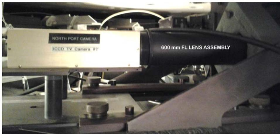
Figure 3: The TV lens assembly after installation. Slide the foam light baffle over the tube.
