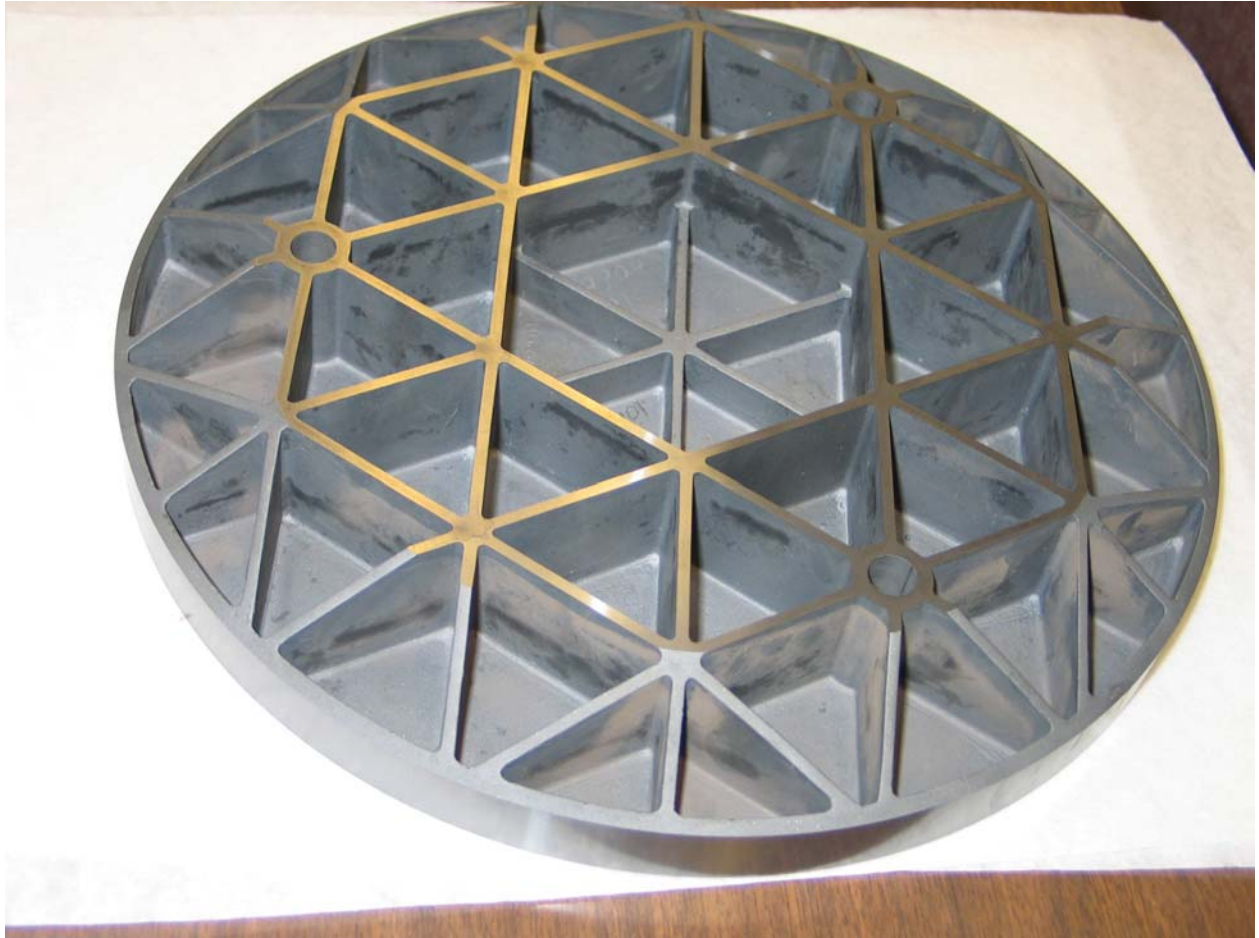
Back surface of a SiC blank manufactured by SSG
