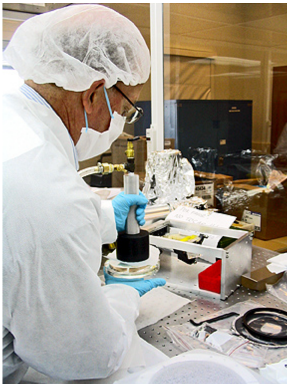
Installing a lens using the NOAO vacuum chuck. This work is done in a "clean room" to prevent contamination of the optics.
