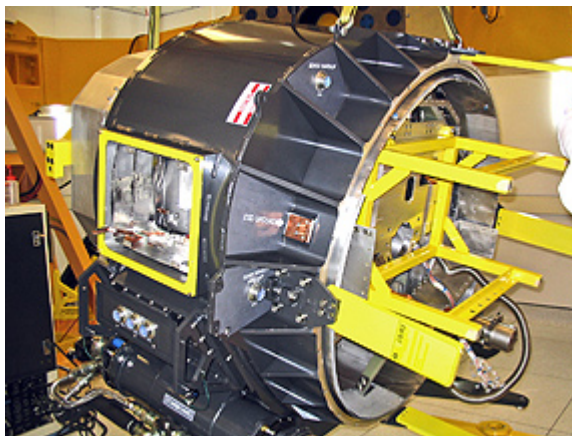
Going back together. The main cold structure is installed in the dewar mid-section. Note the handling fixtures still attached to the dewar shell (right) and cold structure (at both ends).
