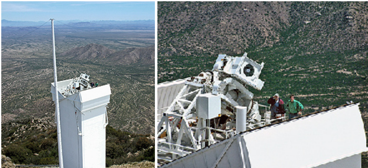
Figure 1. The vector spectromagnetograph mounted on top of the Kitt Peak SOLIS Tower, formerly the vacuum telescope tower. The pole that flanks the tower in the image on the left is part of a lightning protection system. (Photos by Kevin Schramm)
