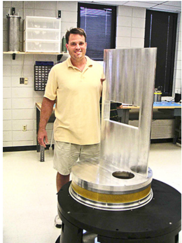
View of the FLAMINGOS-2 camera workbench (top), G-10 spacer, and dewar spacer ring, alongside FLAMINGOS-2 mechanical engineer Jeff Julian.
