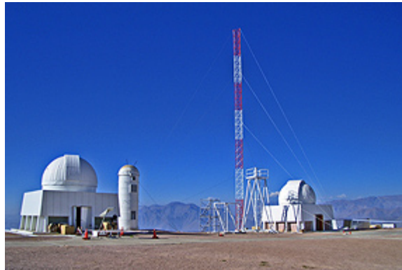
Figure 2. The 30-meter microthermal tower rising above the USNO and Columbia domes on Cerro Tololo. As many as 50+ probes were simultaneously mounted at 10 altitudes on the tower to measure microthermal variations (and hence seeing). The 6.5-meter tower to the right of the 30-meter is the ATST DIMM tower. The tubular tower next to the USNO dome contains the CTIO MASS-DIMM telescope.
