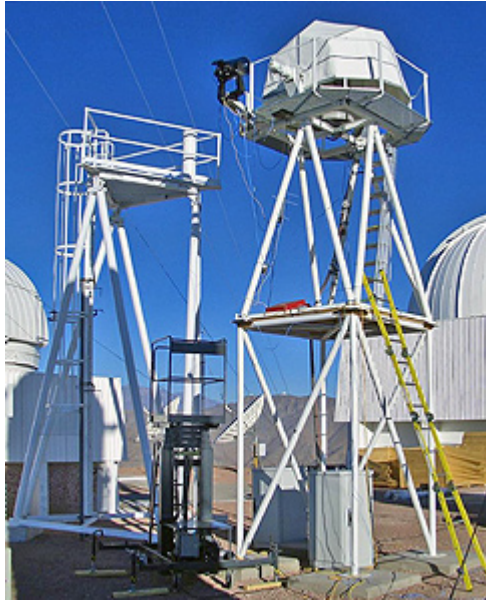
Figure 3. The TMT Halfmann telescope. The 35-centimeter telescope can just be seen through the bottom of the enclosure. The black object to the left on the same tower is a portable Meade telescope/DIMM. The tower to the left is the ATST tower on which the TMT MASS-DIMM telescope will be deployed on remote sites. The final major component of the TMT site testing suite is, of course, the DIMM (deployed as a MASS-DIMM).
