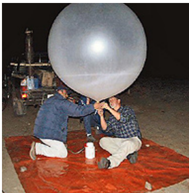
Figure 1. Joselino Vasquez and Gary Poczulp prepare a balloon for launch. The payload consists of sensors and a transmitter/receiver and is carried on a 60-meter tether. The balloons ascend to an altitude of 20–25 kilometers before bursting (with a diameter of ~10 meters).
