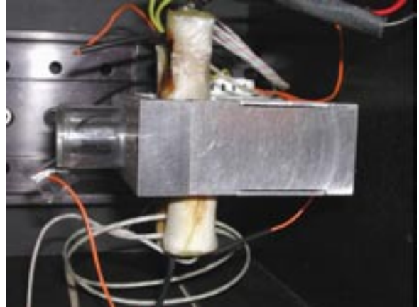
Close-up view of the MOF filter unit mounted at the Hilltop Dome. The quartz container for the sodium vapor protrudes at left center from the magnet housing.
