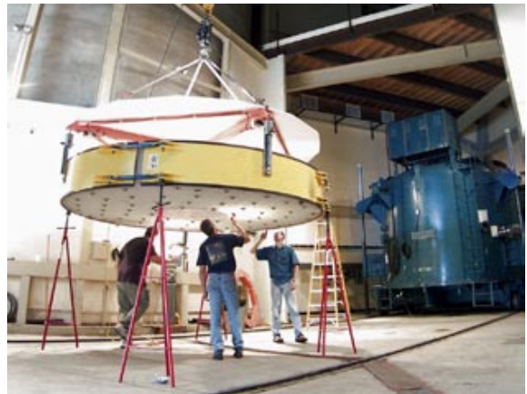
WIYN 3.5-meter mirror being inspected prior to stripping and washing in the upgraded aluminizing area. Note the new location for the vacuum chamber.
