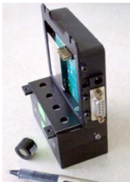
Figure 2. MASS-DIMM installed on a Meade LX200 telescope (left) and its electronics module (right) containing four tiny photomultipliers (one shown apart), photon-counting circuits, and microprocessors.
