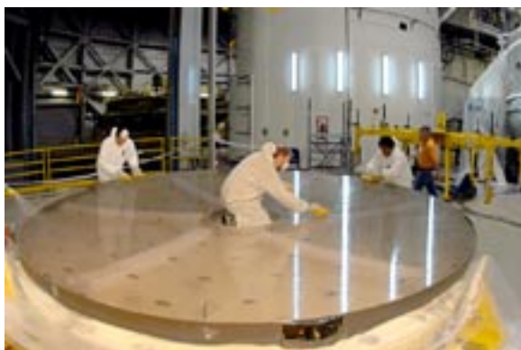
The primary mirror is carefully washed in preparation for aluminization in the Gemini South coating plant.
