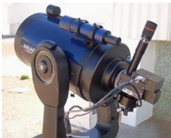
Figure 2. MASS-DIMM installed on a Meade LX200 telescope (left) and its electronics module (right) containing four tiny photomultipliers (one shown apart), photon-counting circuits, and microprocessors.
