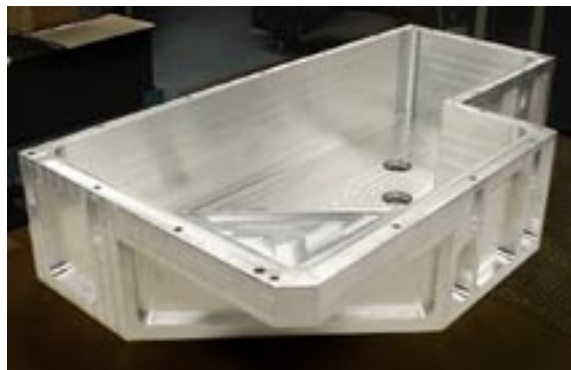
The NICI dewar being fabricated at the machine shop.
