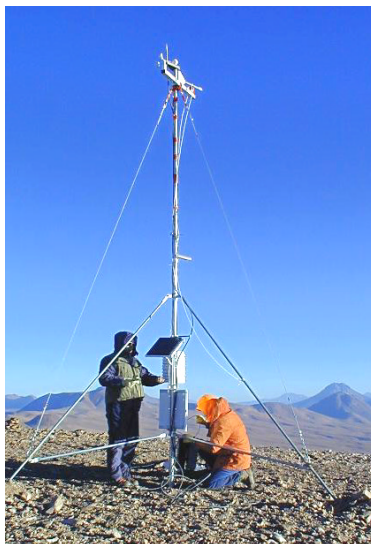
A weather tower was set up over Cerros de Honar to log data over an extended period. Edison Bustos and Brooke Gregory are seen finishing the cabling in late October 2000. (Photo: Bob Blum)
