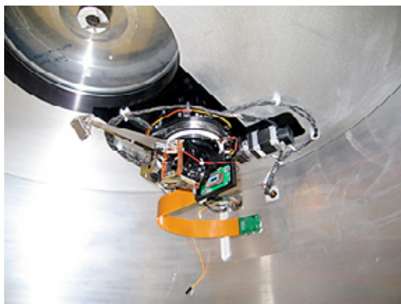
The FLAMINGOS-2 On-Instrument Wavefront Sensor is shown mounted in the dewar.
