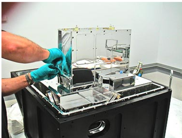
NICI's filter and dichroic wheel assembly is lowered into the NICI dewar prior to the successful cold test.
