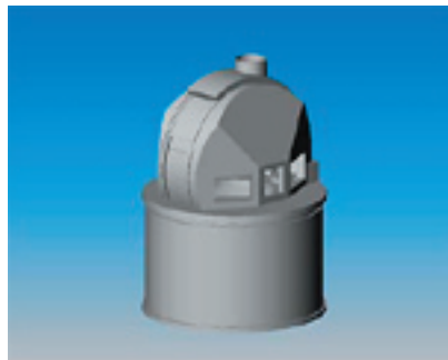
Figure 1. Two ATST enclosure concepts. The left shows a view of the hybrid co-rotating dome. The right is a collapsible dome based upon two facilities built for the US Air Force.
