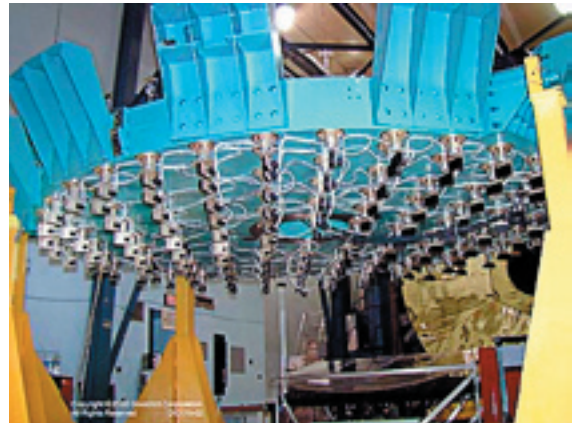
The active support system for the SOAR primary mirror is ready and awaits the completed mirror. One hundred and twenty electromechanical force-feedback actuators support the 4.3 meter diameter, 10 centimeter thin, ULE glass face sheet, and control the correct surface figure as the telescope points around the sky.
