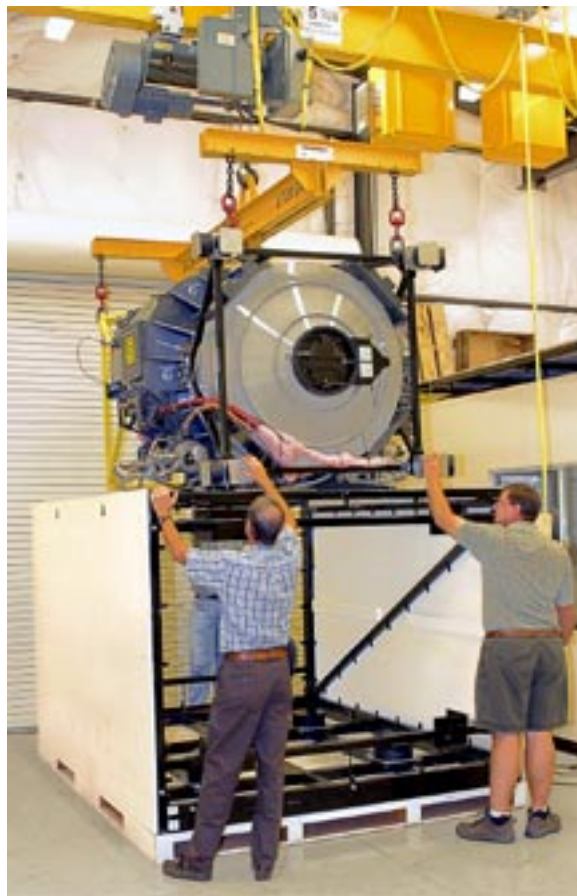
GNIRS is lowered into its crate for shipment to Gemini South under the control of Ron George and the steady hand of Dick Joyce.
