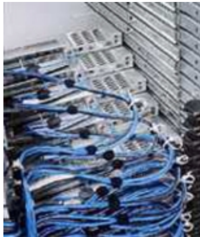
Figure 5. When installed with the Compaq slide rails and cable management solution (left), ProLiant DL360 servers can be fully extended for in-rack service (right).
