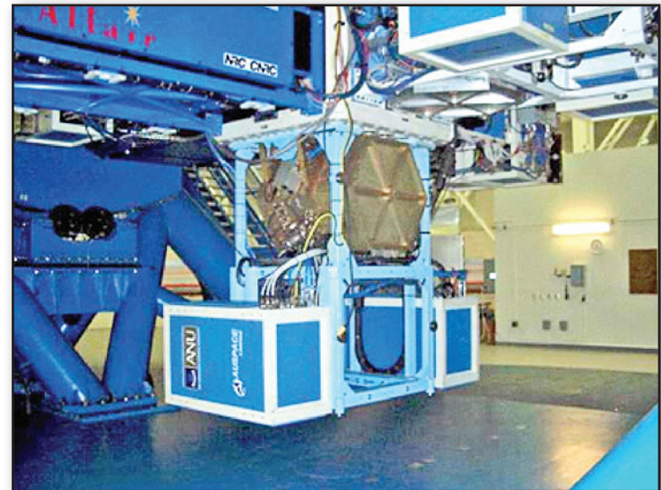
NIFS as deployed on the up-looking port of the Frederick C. Gillett 8-m telescope at Gemini North.
