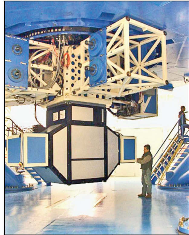
GMOS-S mounted on the up-looking port of Gemini South during instrument commissioning in February 2003
