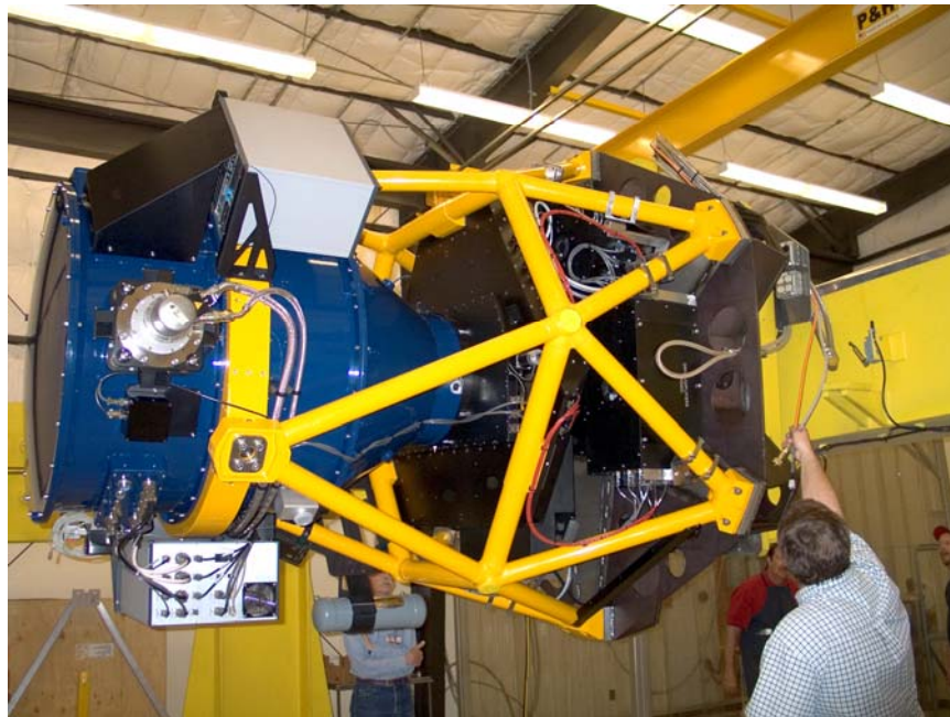
Figure 6: NEWFIRM installed on the NOAO flex rig in February 2006. Team members are connecting the electrical, data and helium service lines prior to startup of the instrument.
